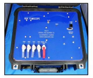
An RDA Fumiscope was also used to measure interior fumigant concentrations during fumigation and initial aeration.
