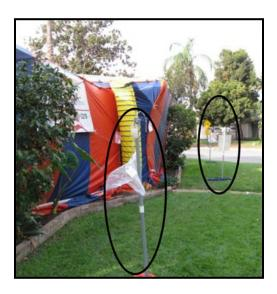
Exterior fumigant concentrations were continuously monitored at eight locations that were evenly spaced and close to the tarp. At each exterior sample location, a calibrated air pump attached to a stand continuously drew air into a gas-tight bag (air sample locations circled).
